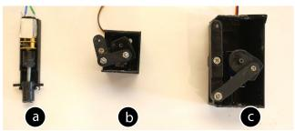
Figure 9: Inside view of a) push actuator, b) wall switch actuator and c) rocker switch actuator.
