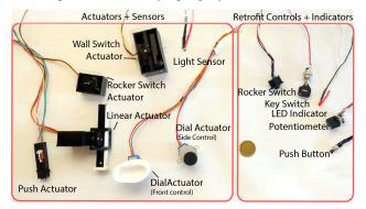
Figure 8: The RetroFab Toolkit; Left) actuators and sensors; the white material of the dial and linear actuator is the parametric component of the design which conforms to the scanned control. Right) controls and indicators.
