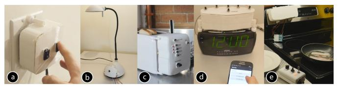
Figure 15: Example retrofit interfaces created using RetroFab: (a) two wall switches, (b) a desk lamp, (c) a toaster, (d) an alarm clock with companion Android application, (e) an oven with remote enclosure.
