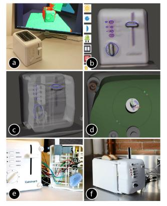
Figure 1: Retrofitting a legacy toaster with RetroFab. (a) The toaster is scanned, (b) the legacy interface is annotated, (c) the attached enclosure is generated, (d) the physical interface and behavior of the retrofit interface is adapted, (e) the enclosure is fabricated and assembled, (f) the new retrofit toaster is perfectly toasting.
