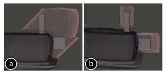
Figure 13: Depending on the surface region covered by the enclosure structure, users can decide to (a) combine actuators in a single enclosure, or (b) group some of them in a separate enclosure structure.
