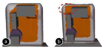
Figure 3: (a) The orange region depicts the enclosure region that RetroFab derives based on the specified components. (b) The user manually extends the region to have additional space for the new shortcut button.
