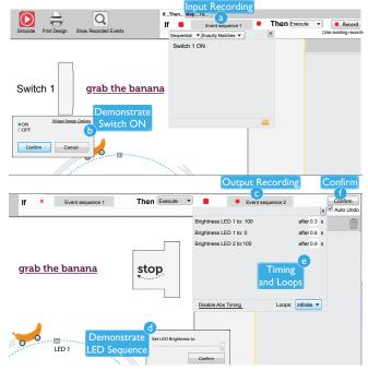
Figure 2. Recording an *if-then* rule for the LED sequence when a switch is turned on.
