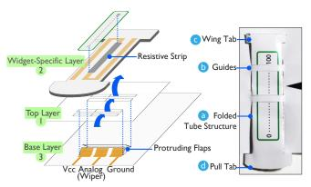
Figure 10. Design of pull-chain widgets: The widget-specific layer is interwoven into the top layer by passing it through four slots. Protruding flaps on the base layer also pass through these slots to ensure constant contact between the winding circuit traces on the pull-chain and the three pin connections on the base layer.
