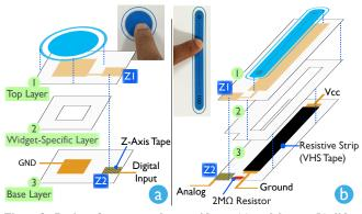
Figure 8. Design of paper-membrane widgets: (a) push button (b) slider.
