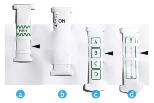
Figure 9. Pull-chain widgets supported by PaperPulse: (a) Push-button, (b) Switch, (c) Radio button, (d) Slider.
