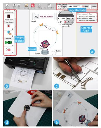
Figure 1. The *PaperPulse* workflow streamlines the entire process of creating interactive paper artifacts. (a) Design and specify logic; (b) print sheets; (c) assemble; (d) upload generated program to microcontroller; (e) final paper artifact.
