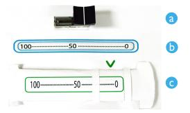
Figure 6. The three families of PaperPulse widgets: (a) Off-the-shelf slider; (b) Paper-membrane slider; (c) Pull-chain slider.
