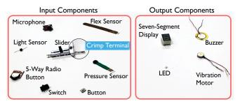
Figure 7. The off-the-shelf widgets currently supported by PaperPulse.
