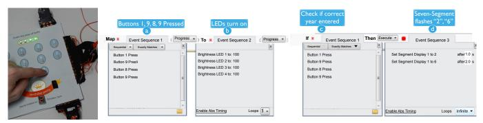
Figure 11. An invitation card with a code slot designed using PaperPulse: (a) Every time the user enters a correct number of the year of birth of the sender, (b) one more LED lights up. (c) When all four numbers are pressed in the right order, (d) the date of the birthday party appears.
