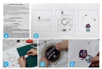
Figure 5. Printing and assembling process: (a) instructions generated; (b) sheets printed (c) circuit and widgets assembled; (d) generated code uploaded to the microcontroller; (e) the final paper artifact.
